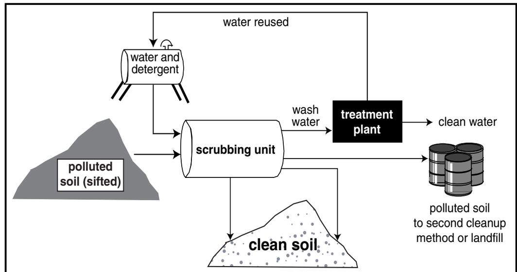
and sometimes detergents, are added to the polluted soil in the scrubbing unit. The mixture of soil and water is passed through sieves, mixing blades, and water sprays. This washes the silt and clay from the larger-grained soil and separates them. Some of the pollution may dissolve in the water or float to the top. The polluted wash water is removed and cleaned up at a treatment plant. The clean water then can be reused in the scrubbing unit or discharged.
